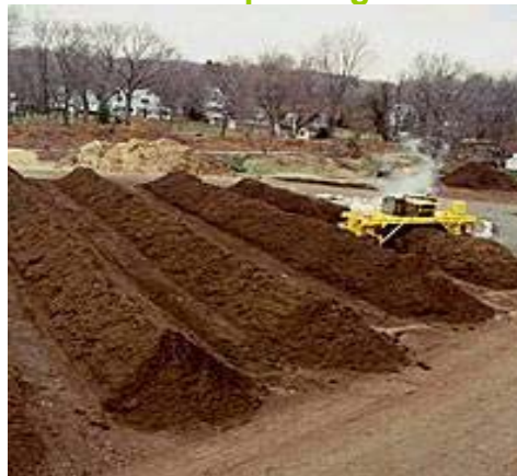
Photo: Windrow composting heaps
